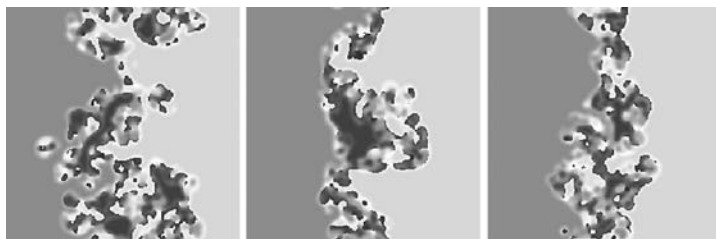
Fig. 28.8. Turbulent fronts separating two homogeneous phases in the 3:1 resonantly forced CGL equation. Reprinted from Hemming and Kapral (2001). Reproduced by permission of The Royal Society of Chemistry.
